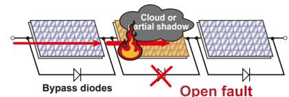
When an open fault occurs, current is forced to flow to the defective cell when it's covered by a shadow, causing the panel to heat up and posing the risk of fire.
