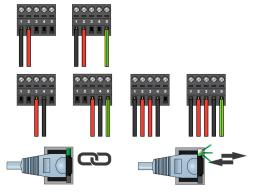
If LED activated there is a network link Wire Size = 26-16 AWG, 0.14mm<sup>2</sup> - 1.3mm<sup>2</sup>
