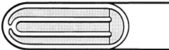
**An earthed (grounded) junction** is also suitable for corrosive media and for high pressure applications. It provides faster response than the insulated junction and protection not afforded by the exposed junction.
