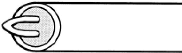
**An exposed (measuring) junction** is recommended for the measurement of flowing or static non-corrosive gas temperature when the greatest sensitivity and quickest response is required.
