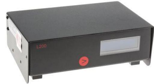
The L200 thermocouple thermometer can be used in conjunction with a PC to provide accurate, versatile 8 channel thermocouple temperature measurement, scanning and logging of measured values. It can also be used as a "stand alone" indicator/logger and incorporates a digital display of measured temperature.
