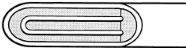
**An insulated junction** is more suitable for corrosive media although the thermal response is slower. In some applications where more than one thermocouple connects to the associated instrumentation, insulation may be essential to avoid spurious signals occurring in the measuring circuits.
