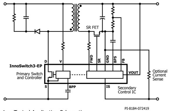
Figure 1. Typical Application Schematic.
