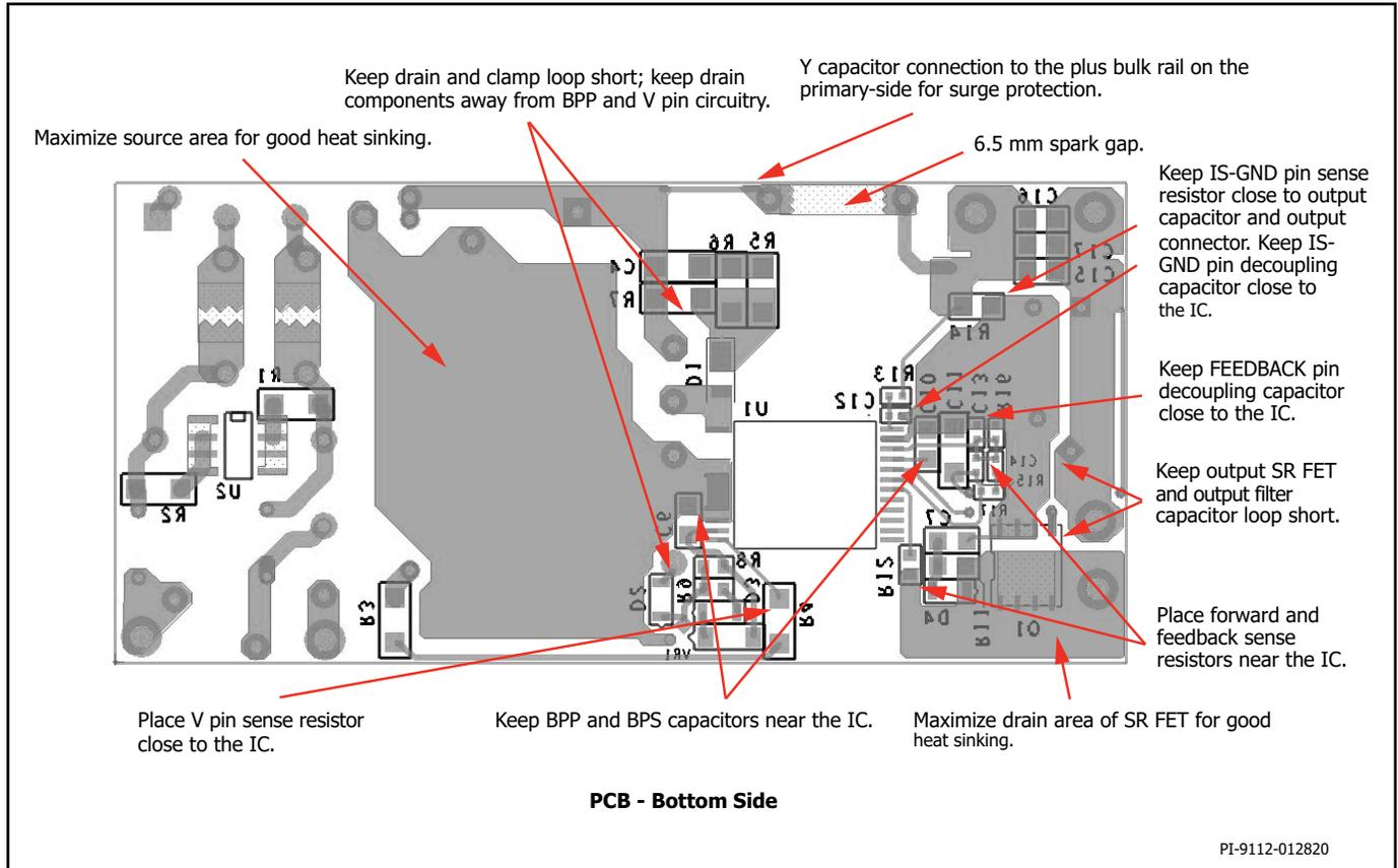
Figure 12. PCB Layout.
