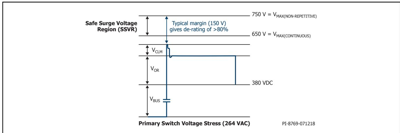
Figure 22. Peak Drain Voltage for 264 VAC Input Voltage.
