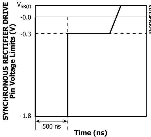
Figure 28. SYNCHRONOUS RECTIFIER DRIVE Pin Negative Voltage.
