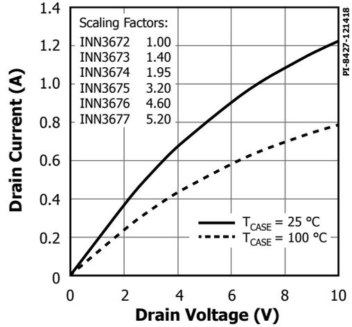
Figure 25. Output Characteristics.
