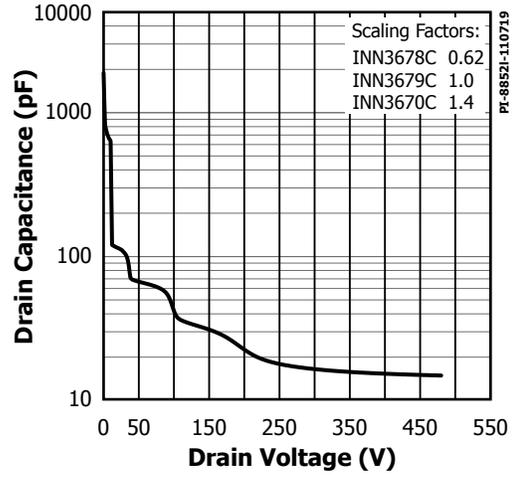
Figure 36. C<sub>oss</sub> vs. Drain Voltage.
