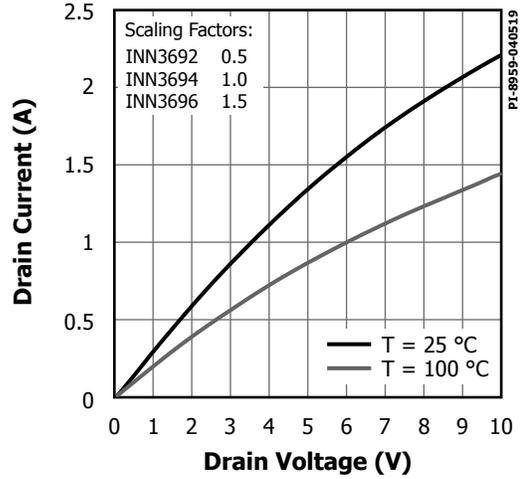
Figure 31. Output Characteristics.
