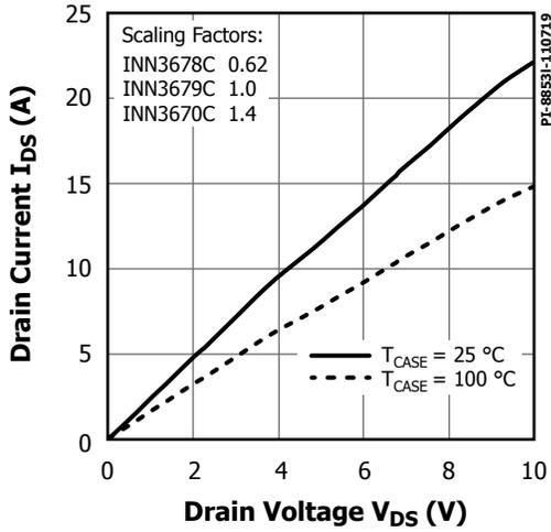
Figure 35. Output Characteristics.
