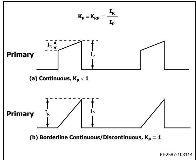
Figure 20. Continuous Conduction Mode Current Waveform,  $K_p < 1$ .
