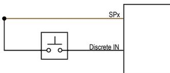
Discrete Input Wiring for NPN Sensors
