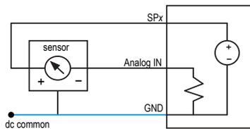
Thermistor Input Wiring
