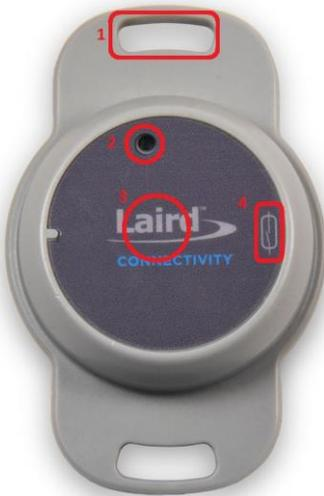
**Figure 3: Front side of the Sentrius™ BT510 sensor**
