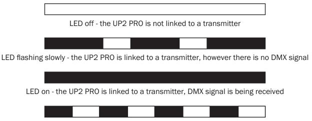
LED flashing fast - the UP2 PRO is trying to establish a connection/connection has been lost
