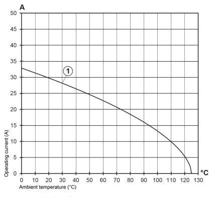
① Conductor cross-section 2.5 mm<sup>2</sup> Current rating of the Han  $E^{\textcircled{R}}$  contacts
