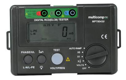
This is mainly used to detect whether the RCD in the circuit can be triggered normally. It is only suitable for single-phase circuits with the supply voltage range of 195V to 253V. Its voltage measurement range is 30V to 600V, 45Hz to 65Hz.
