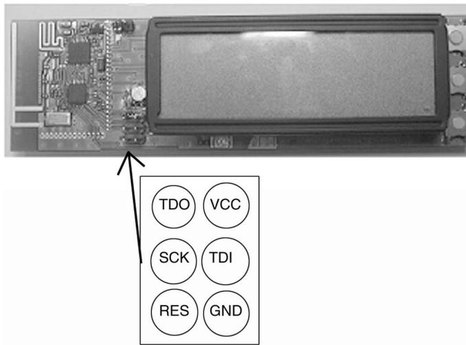
AVRStudio can be downloaded from the Atmel web site at no cost. The 2 x 3 connector at the bottom of the reference design board is used to flash and debug the AVR microcontroller. The connection between the reference design board and AVRStudio is realized by the JTAG MK 2 connected to the 2 x 3 connector, using a the squid cable included in the JTAG MK 2 ([Figure 12-2 on page 13](#)).
