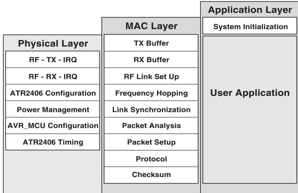
The RF firmware implements three main layers to set up the RF link and to exchange data via RF. The lowest layer (the physical layer) is responsible for the exchange of the RF data and the configuration of the ATR2406. The second layer (the MAC layer) handles the transmit and receive buffers, holding the RF data. The MAC layer also generates the timing needed to control the RF chip, and analyzes the received packet and the setup of a response packet.
