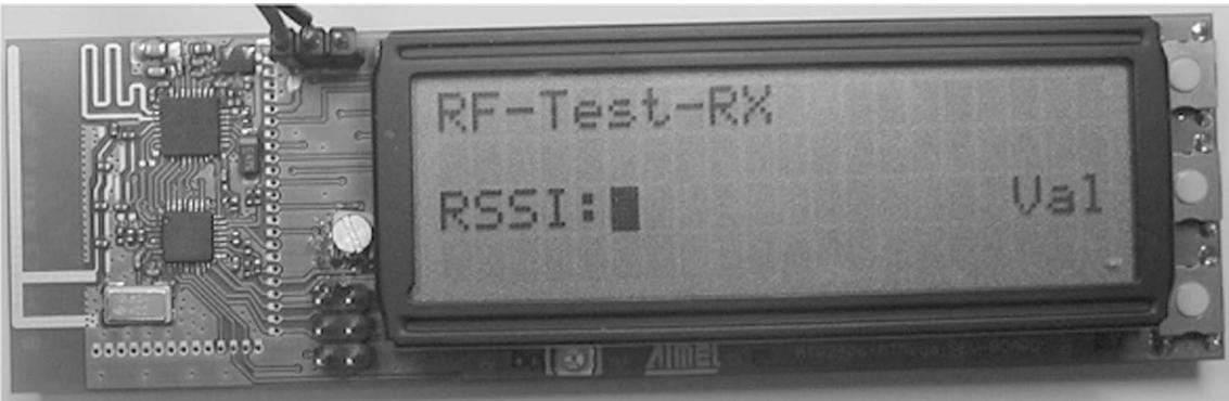
Figure 12-20. RF-Test-RX Value Selection Menu, Signal Present
