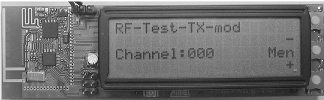
**Figure 12-10.** RF-Test-TX-mod Channel Selection Menu
