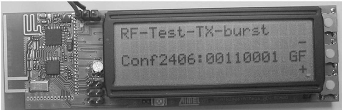
**Figure 12-16.** RF-Test-TX-burst Channel Selection Menu
