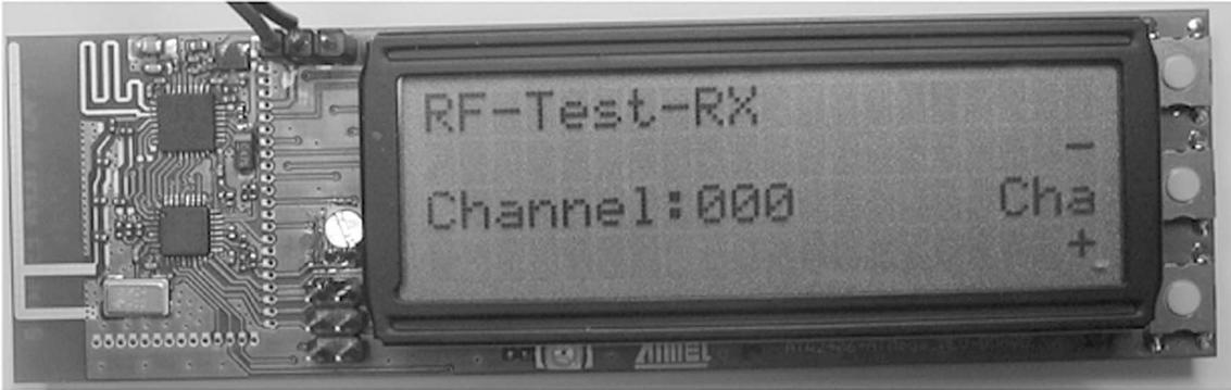
Figure 12-19. RF-Test-RX Value Selection Menu, No Signal Present
