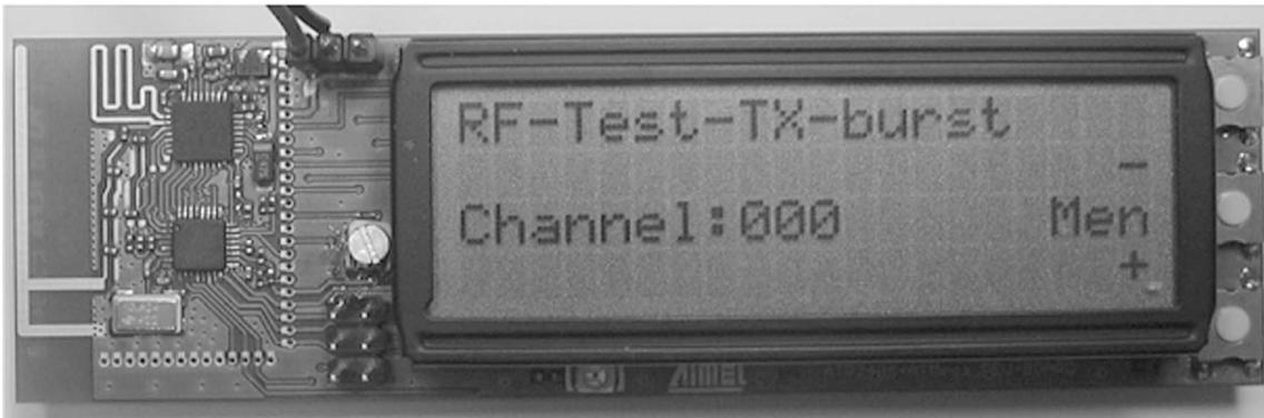
**Figure 12-14.** RF-Test-TX-burst Hopping Selection Menu
