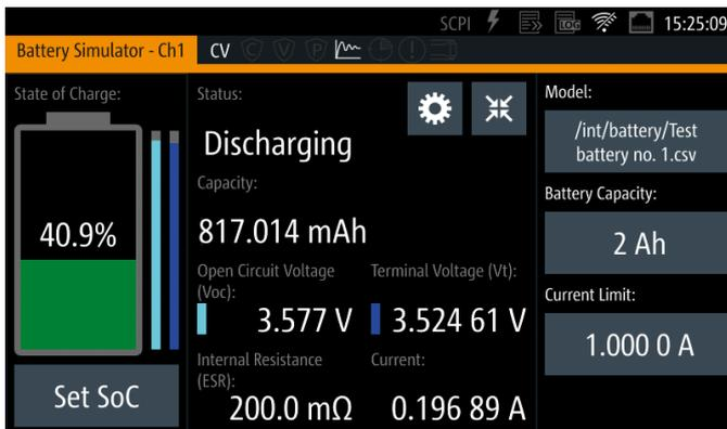
The battery simulation software includes data sets of common battery types that can be easily modified.
