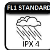
Water Resistant IPX4 – works after splashing water on all sides
