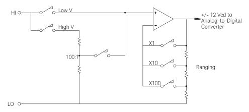
For input voltages less than 12 VDC, the **Low V** switch is closed and applies the input signal directly to the input amplifier. For higher voltages, the **High V** switch is closed and the signal is attenuated 100:1 before being applied to the input amplifier. The input amplifier gain is set to one of three values (x1, x10, or x100) to yield a signal in the range of  $\pm 12$  VDC for the analog-to-digital converter.
