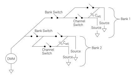
If you are not using all of the channels on the multiplexer, divide the input signals equally between Bank 1 and Bank 2. For example, if you are multiplexing eight channels using the 16-channel multiplexer, use four channels in the lower bank and four channels in the upper bank. For even better noise immunity, leave one unused, grounded channel between each input channel.
