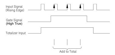
Using the hardware jumper labeled "Totalize Threshold" on the module, you can control the threshold at which an edge is detected. Move the jumper to the "AC" position to detect changes through 0 volts. Move the jumper to the "TTL" position (factory setting) to detect changes through TTL threshold levels.
