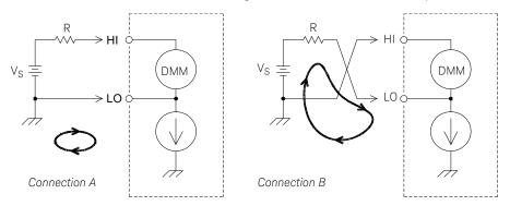
The measurement noise caused by injected current can be significantly reduced by setting the integration time of the internal DMM to 1 PLC or greater (see page 133 for a discussion of integration time).
