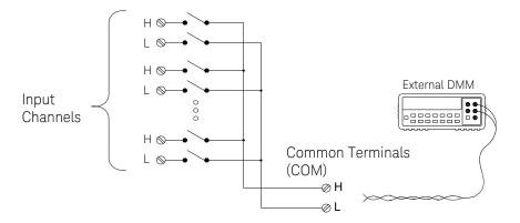
To control scanning with an external instrument, two control lines are provided. When the 34970A/34972A and the external instrument are properly configured, you can synchronize a scan sequence between the two.
