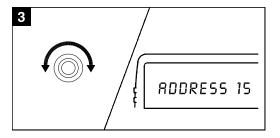
**3** Rotate the knob to view the choices on this level of the menu. When you reach the end of the list, rotate the knob in the opposite direction to view all of the other choices.
