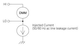
With *Connection A* (see below), the injected current flows from the earth connection provided by the circuit to the LO terminal of the internal DMM. This configuration adds no noise to the measurement. However, with *Connection B*, the injected current flows through the resistor R thus adding noise to the measurement. With Connection B, larger values of R will make the problem worse.
