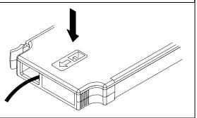
5 Install the module into mainframe.
