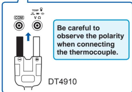
**When measuring temperatures with the thermocouple applied to the surface of the measurement object**
