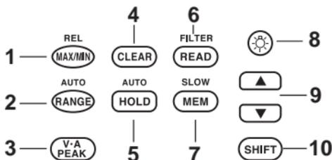
(\*) Pressing a key **for at least 1 second** activates the function indicated above the key. To disable the function, change the rotary switch setting.
