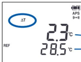
When measuring temperature, [REF] lights up and a standard temperature appears in the sub display.
