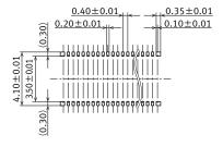
Recommended metal mask pattern Metal mask thickness: When 120 μm (Opening ratio: 40%)
