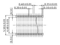
Recommended metal mask pattern Metal mask thickness: When 120 μm (Opening ratio: 50%)
