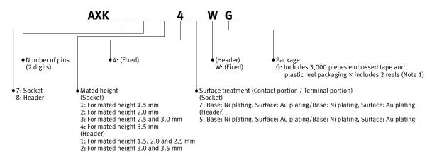
Note: 1. Only a socket of mated height 3.5 mm: 2,000 pieces embossed tape and plastic reel packaging  $\times$  2 reels
