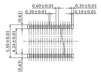
■ Keep the PC board warp no more than 0.03 mm in relation to the overall length of the connector.
