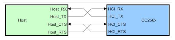
When the UART Rx buffer of the CC2564C passes the "flow control" threshold, it will set the signal UART\_RTS high to stop transmission from the host.
