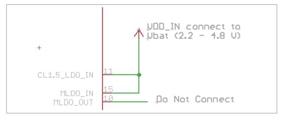
Full-DC2DC system (Lower RF output power, but optimum system power):
