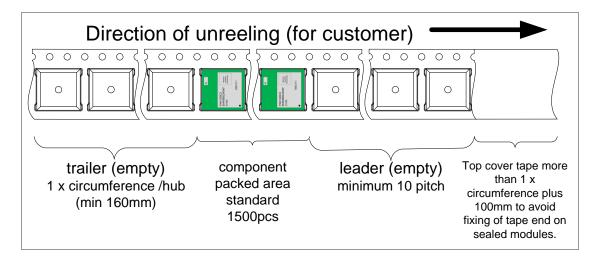
Empty spaces in the component packed area shall be less than two per reel and those spaces shall not be consecutive.
