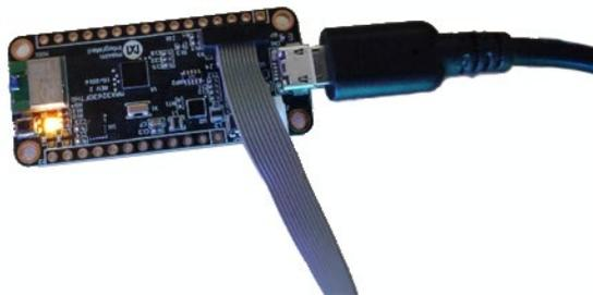
Figure 8. MAX32630FTHR host blinking LED.
