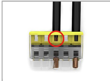
The transparent housing shows if conductors are fully inserted; within the colored base, a clear port shows if the conductor's strip length is correct. Conductors are correctly stripped if the clear port shows no bare conductor on the unprinted connector side. Picture shows center conductor with exceeded strip length.
