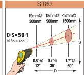
Use the ST80/ST80-IS within 8m (25 feet) of the intended target. At greater distances, the measured area will be larger (approximately the distance divided by 50).
