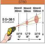
Use the ST60 within 5m (15 feet) of the intended target. At greater distances, the measured area will be larger (approximately the distance divided by 30).
