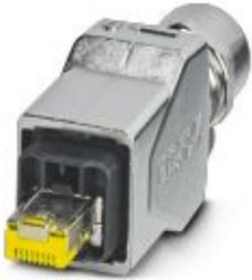
Push-pull ADVANCE connector (version 14), die-cast zinc, with RJ45 connector insert, 8-pos., 10 Gbps, CAT6<sub>A</sub> (IEC 11801:2017), with IDC fast connection technology, for AWG 23 - 22 1-wire, 7-wire, and 19-wire conductors, for cable diameter of 5.5 mm ... 10 mm
