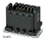
SMD male connector, Nominal current at 20 °C: 1.7 A, Test voltage: 500 V AC, number of positions: 12, pitch: 0.8 mm, color: black, contact surface: Gold
