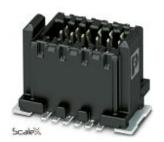
SMD male connector, Nominal current at 20 °C: 1.7 A, Test voltage: 500 V AC, number of positions: 20, pitch: 0.8 mm, color: black, contact surface: Gold
