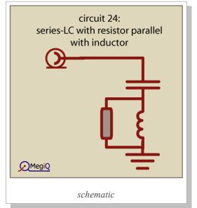
At very high frequency the capacitor has a very low impedance and the inductor a very high one, so the  $50\Omega$  of the resistor dominated the graph at high frequencies.
