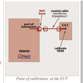
The instrument stores this set of calibration data, and since the MegiQ VNA is very temperature stable, you will not have to perform this calibration routine very often.
