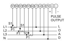
It is recommended that all voltage lines are fitted with 1 Amp HRC fuses. For safety reasons, CT secondary connections should be grounded according to local codes of practice.
