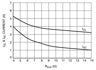
Figure 3. Current Limit vs. R<sub>limit</sub> for Direct Current Sensing
