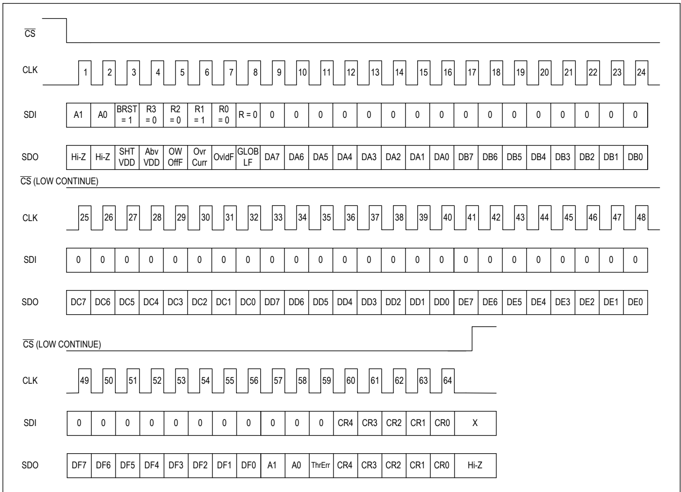
Figure 15. SPI Burst Read with CRC Enabled
