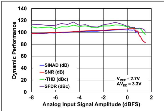
**FIGURE 2-19:** Dynamic Performance vs. Input Signal Amplitude.
