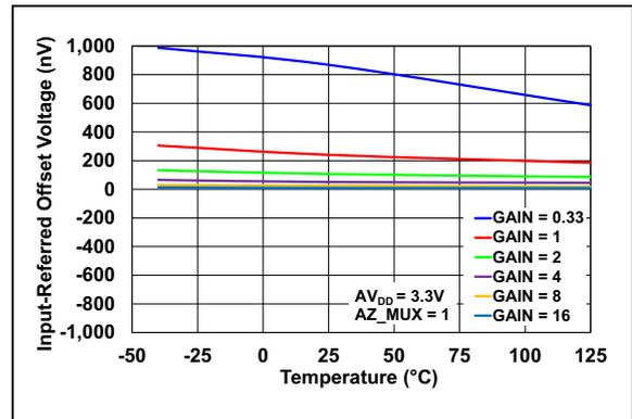
**FIGURE 2-29:** Offset Error vs. Temperature ( $AZ\_MUX = 1$ ).
