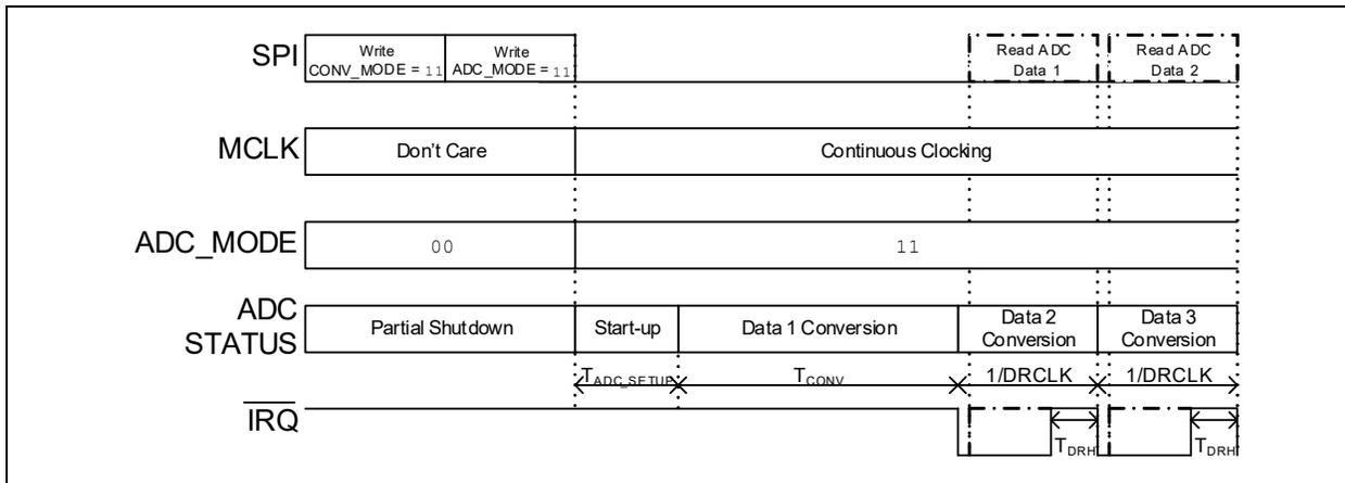
FIGURE 5-14: MUX Continuous Conversion Mode Timing Diagram.
