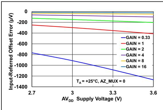
**FIGURE 2-26:** Offset Error vs.  $AV_{DD}$  ( $AZ\_MUX = 0$ ).
