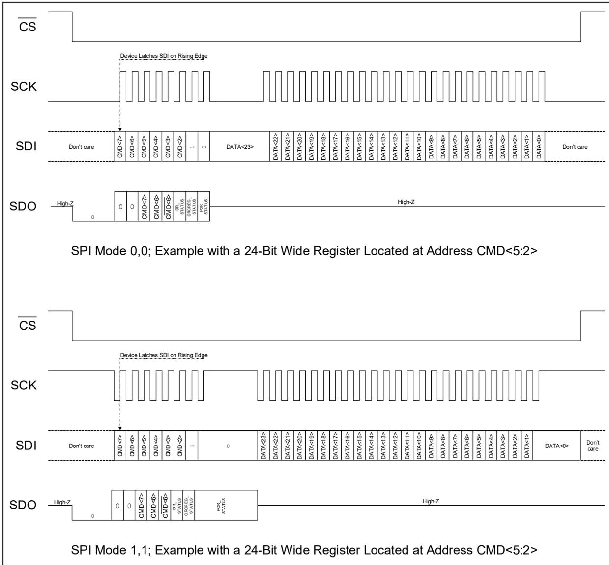
**FIGURE 6-4:** Single Register Write Communication (CMD[1:0] = 10) Timing Diagram.
