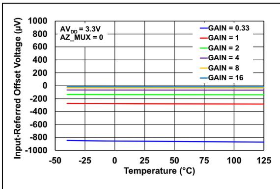
**FIGURE 2-27:** Offset Error vs. Temperature ( $AZ\_MUX = 0$ ).
