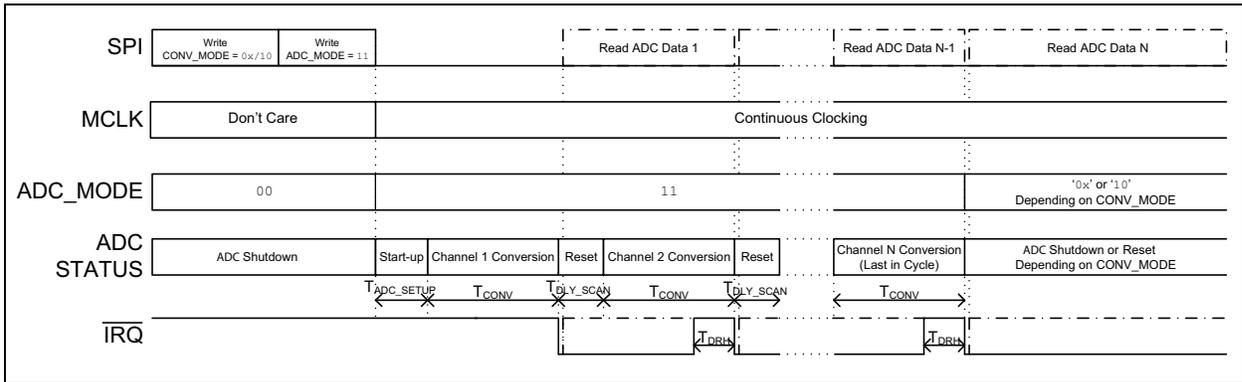
**FIGURE 5-15:** SCAN One-Shot Conversion Mode Timing Diagram.
