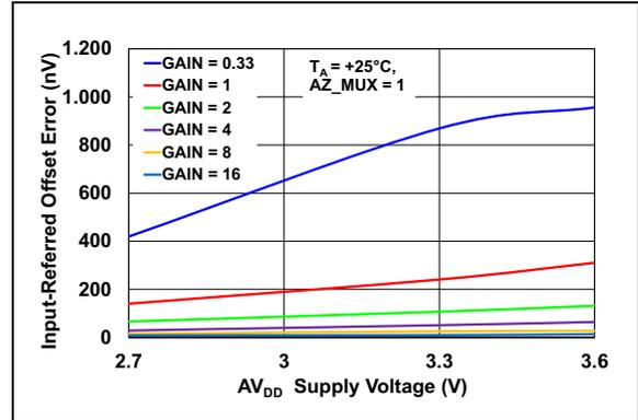
**FIGURE 2-28:** Offset Error vs.  $AV_{DD}$  ( $AZ\_MUX = 1$ ).
