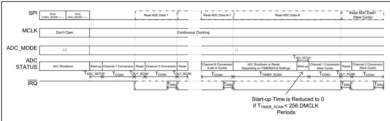
**FIGURE 5-16:** SCAN Continuous Conversion Mode Timing Diagram.
