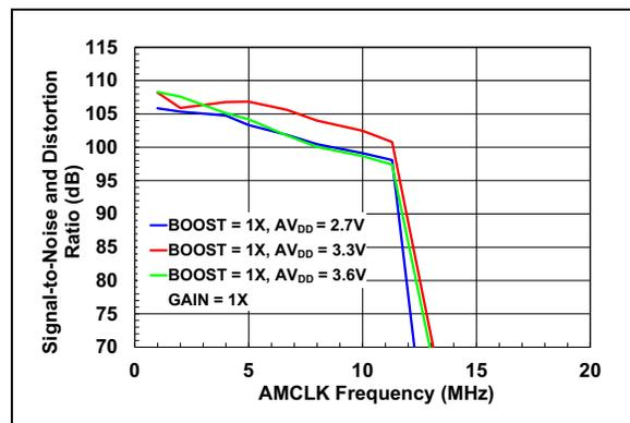
**FIGURE 2-24:** SINAD vs. AMCLK vs.  $V_{DD}$ .
