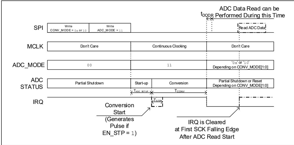
FIGURE 5-13: MUX One-Shot Conversion Mode Timing Diagram.
