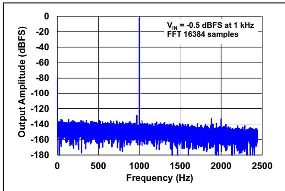
**FIGURE 2-2:** FFT Output Spectrum,  $f_{in} = 1\text{ kHz}$ .
