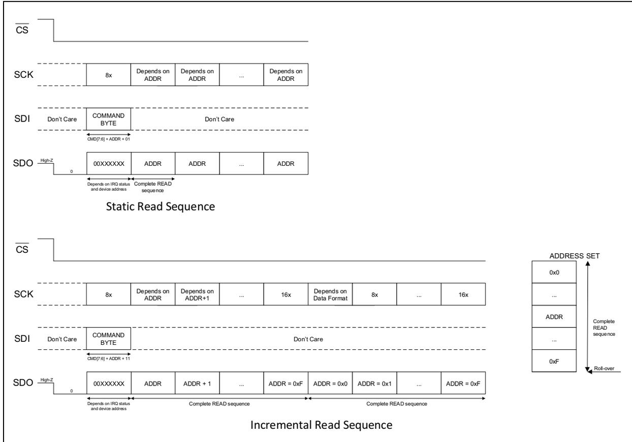
**FIGURE 6-8:** Static and Incremental Read SPI Communications.
