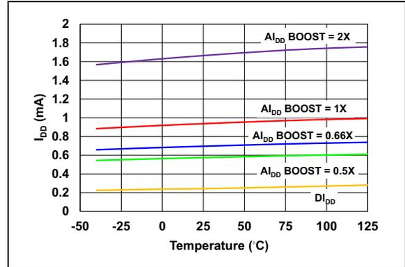
**FIGURE 2-38:**  $D I_{DD}$  and  $A I_{DD}$  vs. Temperature.
