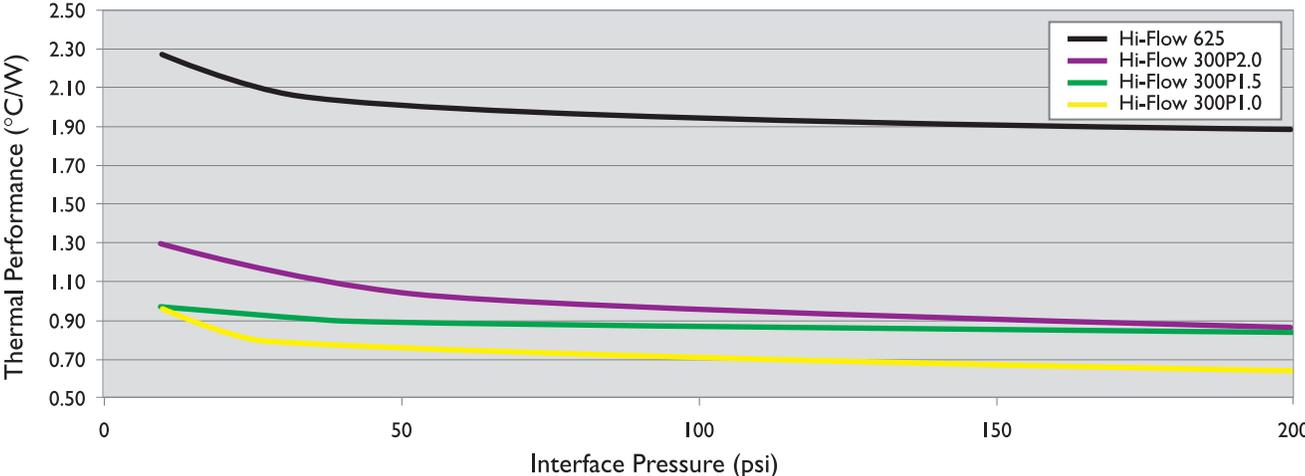
Non-Isolating Hi-Flow Series 105 to 300 Grease Replacement Materials
