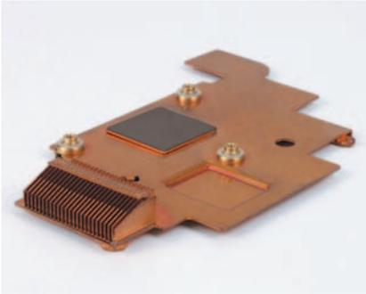
Hi-Flow 225UT is designed as a pressure sensitive thermal interface material for use between a high performance processor and a heat sink. Hi-Flow 225UT is a thermally conductive 55°C phase change composite with inherent tack. The material is supplied on a polyester carrier liner and is available with high-visibility protective tabs.
