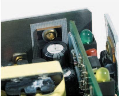
Sil-Pad 400 is a composite of silicone rubber and fiberglass. The material is flame retardant and is specially formulated for use as a thermally conductive insulator. The primary use for Sil-Pad 400 is to electrically isolate power sources from heat sinks.
