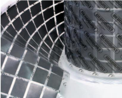
Gap Pad I500R has the same highly conformable, low-modulus polymer as the standard Gap Pad I500. The fiberglass reinforcement allows for easy material handling and enhances puncture, shear and tear resistance. The natural tack on both sides of the material allows for good compliance to mating surfaces of components, further reducing thermal resistance.
