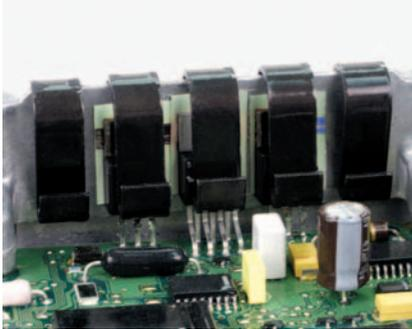
Bergquist Sil-Pad AI500 is a silicone-based, thermally conductive and electrically insulating material. It consists of a cured silicone elastomeric compound coated on both sides of a fiberglass reinforcement layer.
