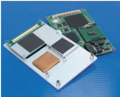
Gap Pad I500 has an ideal filler blend that gives it a low-modulus characteristic that maintains optimal thermal performance yet still allows for easy handling. The natural tack on both sides of the material allows for good compliance to adjacent surfaces of components, minimizing interfacial resistance.
