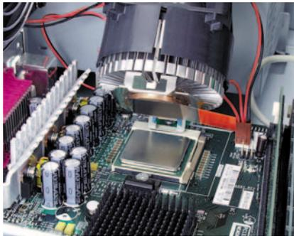
Hi-Flow 225U is designed for use as a thermal interface material between a computer processor and a heat sink. The product consists of a thermally conductive 55°C phase change compound coated on a release liner and supplied on a carrier.
