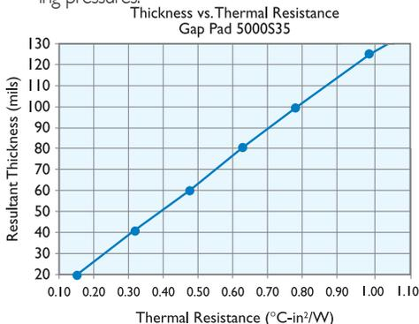
Note: Resultant thickness is defined as the final gap thickness of the application.
