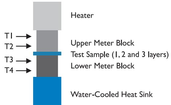
2 in. diameter stack (ref. 3.14 in<sup>2</sup>) – 10-500 psi, 1 hour per layer
