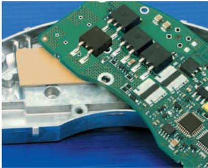
Gap Pad A3000 is a thermally conductive, filled-polymer laminate, supplied on a reinforcing mesh for added electrical isolation, easy material handling and enhanced puncture, shear and tear resistance. Gap Pad A3000 has a reinforcement layer on the dark gold side of the material that assists in burn-in and rework processes while the light gold and soft side of the material allows for added compliance.
