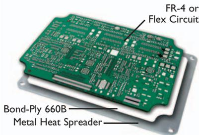
Bond-Ply 660B is a thermally conductive, electrically insulating, double-sided pressure sensitive adhesive tape. The tape consists of a high performance, thermally conductive acrylic adhesive coated on both sides of a PEN film. Use Bond-Ply 660B in applications to replace mechanical fasteners or screws.
