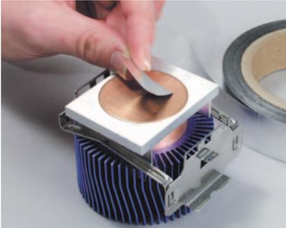
Bergquist reworkable Hi-Flow 225FT thermal interface material provides a low thermal resistance path between hot components such as high performance processors and heat sinks. The material consists of a 55°C phase change compound bonded to one side of a conformable metal foil. This pressure sensitive material is easily applied to the heat sink and securely conforms to many mounting surfaces. Its compliant foil allows for easy release and reworking without leaving residue on CPU surfaces.
