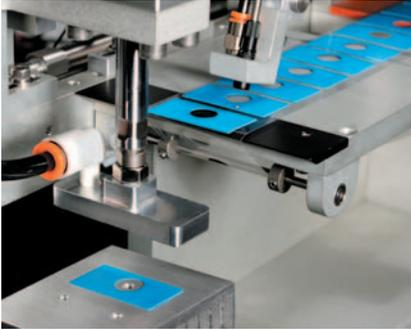
Bergquist Sil-Pad I500ST (Soft Tack) is a fiberglass reinforced thermal interface material that is naturally tacky on both sides. Sil-Pad I500ST exhibits superior thermal performance when compared to the competitors' thermal interface materials. Sil-Pad I500ST is supplied in sheet or roll form for exceptional auto-dispensing and auto-placement in high volume assemblies. Sil-Pad I500ST is intended for placement between an electronic power device and its heat sink.
