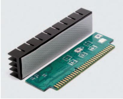
Gap Pad A2000 acts as a thermal interface and electrical insulator between electronic components and heat sinks. In the thickness range of 10 to 40 mil, Gap Pad A2000 is supplied with natural tack on both sides, allowing for excellent compliance to the adjacent surfaces of components. The 40 mil material thickness is supplied with lower tack on one side, allowing for burn-in processes and easy rework.
