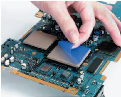
Gap Pad 2500 is a thermally conductive, electrically insulating, unreinforced gap filling material. Gap Pad 2500 is a filled-polymer material yielding an elastic polymer that allows for easy handling and converting without the need for reinforcement. These properties also allow for good wet-out and interfacing characteristics to surfaces with roughness and/or topography. All these characteristics make this material ideal for applications using either clip or screw-mounted assemblies.
