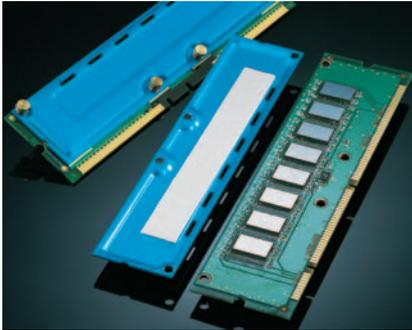
Gap Pad HC 1000 is an extremely conformable, low-modulus polymer that acts as a thermal interface and electrical insulator between electronic components and heat sinks. The “gel-like” modulus allows this material to fill air gaps to enhance the thermal performance of electronic systems. Gap Pad HCI000 is offered with removable protective liners on both sides of the material.
