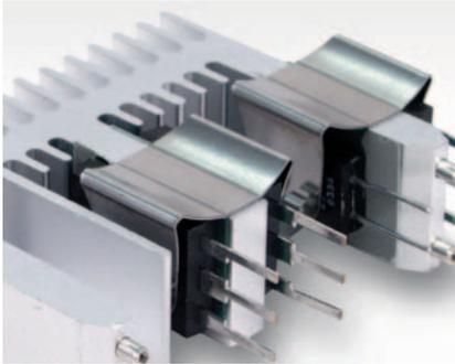
Bergquist Hi-Flow I15-AC is a thermally conductive fiber reinforced phase change material. The product consists of a thermally conductive 65°C phase change compound coated on a fiberglass web, and an adhesive coating on one side for attachment to a cold heat sink. There is no need to preheat the heat sink to apply the Hi-Flow I15-AC.
