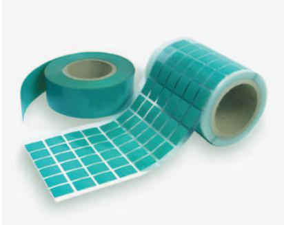
Hi-Flow 300G consists of a thermally conductive 55°C phase change compound coated on a fiberglass web. Hi-Flow 300G is designed as a thermal interface material between a computer processor and a heat sink.
