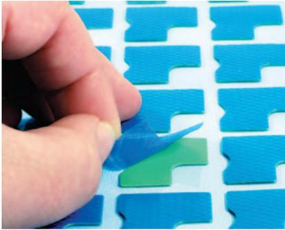
The new Gap Pad I000SF is a thermally conductive, electrically insulating, silicone-free polymer specially designed for silicone-sensitive applications. The material is ideal for applications with high standoff and flatness tolerances. Gap Pad I000SF is reinforced for easy material handling and added durability during assembly. The material is available with a protective liner on both sides of the material.
