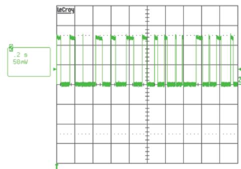
For the EVS system WERMA employs light emitting diodes. A micro-processor generates random light signals. This gives the light a very "agitated" character which proves highly effective in drawing the attention of those in its vicinity – even when seen out of the corner of the eye.
