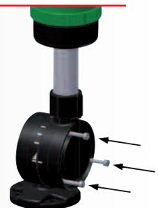
Secure the two parts with the screws supplied
