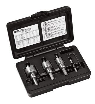
This 4-piece Carbide-Tipped Hole Cutter kit cuts quick, precise holes in a variety of materials. Set includes three commonly used sizes plus an extra pilot bit. Integrated flange prevents the operator from drilling beyond the sheet metal. Split point pilot drill bit prevents bit walking.
