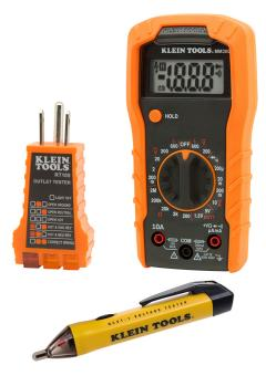
Klein Tools Multimeter Test Kit contains MM300 (Manual-Ranging digital Multimeter), NCVT-1 (Non-Contact Voltage Tester) and the RT105 (Receptacle Tester). The NCVT-1 automatically detects standard voltage in cables, cords, circuit breakers, lighting fixtures, switches, outlets, and wires. The RT105 detects the most common wiring problems in standard receptacles.
