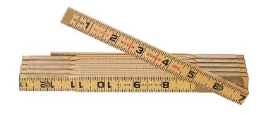
Klein Tools Wood Folding Rules are constructed of strong, 6-foot (1.83 m) long hardwood with a clear-abrasion-resistant coating for added protection on the jobsite. The black measurement markings stand out against the yellow background for easier reading. There are black markings on yellow, with red stud center markings every 16 inches (406.4 mm).
