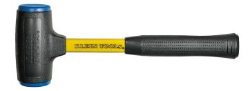
The Klein Tools Dead Blow Hammer has 40-Percent more driving power than other dead blow hammers. When struck, the shot directs the striking power and increases the impact, creating a dead blow effect. The reduced rebound upon impact transfers the full energy of the blow to the object being struck.
