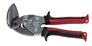
Klein Tools' Upright Snips cut straight, curves, and tight circles in 24 gauge cold rolled steel and 28 gauge stainless steel. This tool makes cutting easier in confined spaces (in ductwork, reaching through openings or against a wall). Soft touch aviation grips provide maximum control and comfort. The blades are made of long-lasting serrated forged steel for superior strength and durability. Tip-Ident® on the handles and color-coding allow for easy identification of the cutting pattern.
