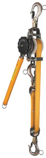
Klein Tools' Web-Strap Ratchet Hoist with hot rings to accommodate hotsticks. The hoist features a tighter ratchet to reduce work and fatigue. The handle and drum knob allow you to safely control the tension release to avoid free wheeling. The hoist can be used in both a single line and double line configuration. The handle provides a 360-degree range of motion for easier adjustment from any angle.
