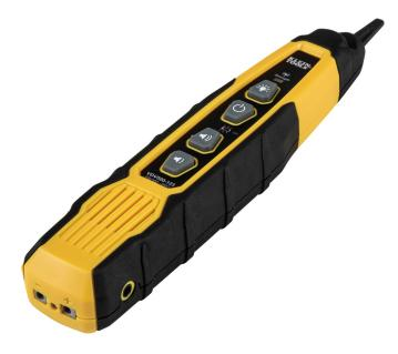
The professional series Probe-Pro Tone Tracer traces non-active wiring when used with Toner-Pro Tone Generator (VDV500-063, sold separately). It features a responsive, durable, replaceable non-metallic, conductive tip and a work light for use in dark spaces. A headphone jack allows for headphone (not included) use in extreme noise environments. The terminal block confirms the toned pair has been located.
