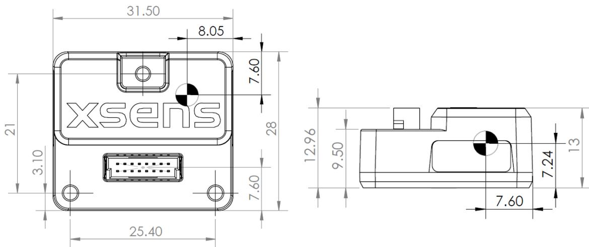
Figure 5: Location origin of measurements (dimensions in mm)
