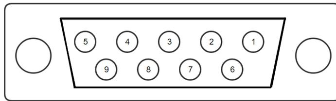
Figure 8: Pin out of DSUB9 connector CAN
