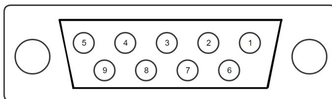
Figure 9: Pin out of DSUB9 connector RS232
