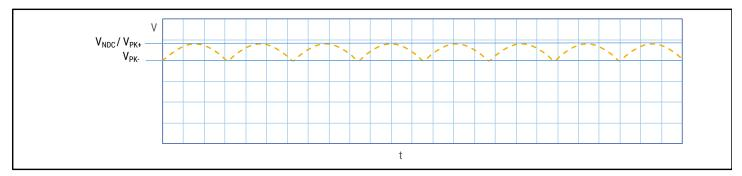
The applied peak-to-peak ripple voltage shall not exceed 0.1 x  $V_{\text{NDC}}$ . The peak voltage shall not exceed the rated voltage  $V_{\text{NDC}}$ .
