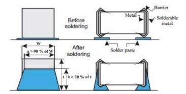
Figure 4: Soldering Criterion in case of Wave and IR Reflow Pb-containing Soldering
