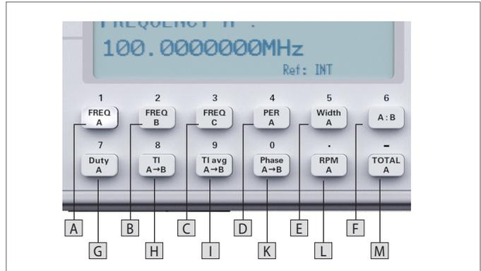
Fig. 3.1: The function keys and their meaning
