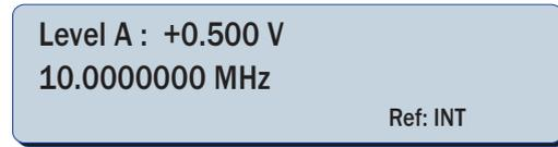
Optimum triggering is obtained by setting the trigger level to about 50 % of the peak-to-peak amplitude of the input signal. In manual mode proper triggering can be checked by the trigger indicators [19] and [23] control of channels A [20] and B [22] as follows:
