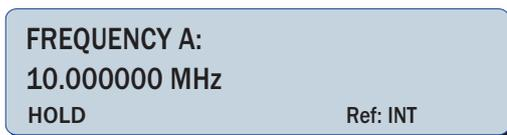
By pressing the pushbutton OFFSET [29] the Offset function will be activated, the pushbutton OFFSET [29] will light up. In this mode the present result will be taken as the reference value and indicated in the display (e.g. REF: 100.000000 MHz). For all subsequent measurements this value will be subtracted from the result, the difference will be displayed.
