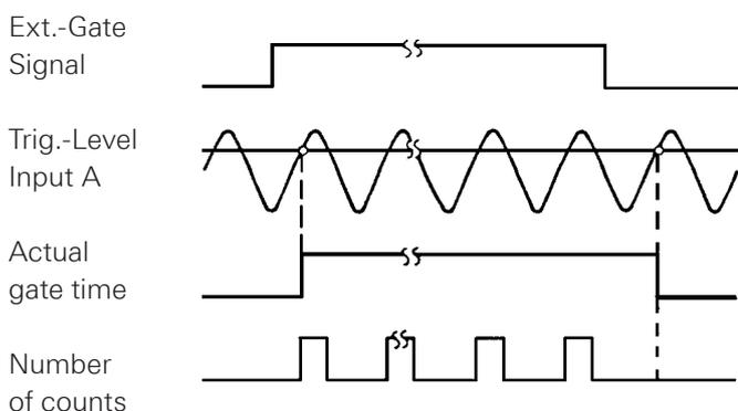
A measurement may be started and stopped by a signal at the gate input TRIG/ARM [32]. This input is located on the front panel. The gated mode is entered by pressing GATED [30], the pushbutton will light up. As long as there is a low level at this input no measurement will be started. A measurement is started by a low to high transition at the TRIG/ARM input [32] and if the trigger conditions are met.
