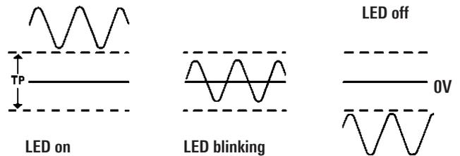
Suitable setting of the attenuators [13] and [18] is a prerequisite for correct measurements. With too much attenuation the residual noise of the input signal comparator will affect the result. With too little attenuation or if the input signal is too large the input stage may be overdriven which lead to erroneous measurements.
