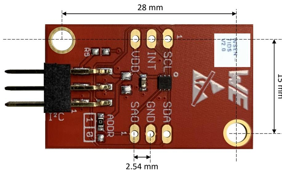
Figure 1: Evaluation board for the temperature sensor IC
