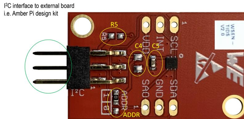
Figure 2: Pin header connection to the external boards. e.g. Amber Pi design kit
