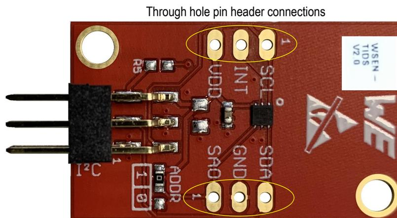
Figure 3: Through hole connection
