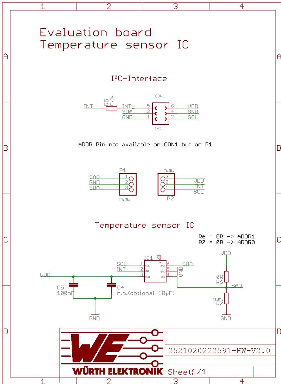
Figure 4: Schematic diagram
