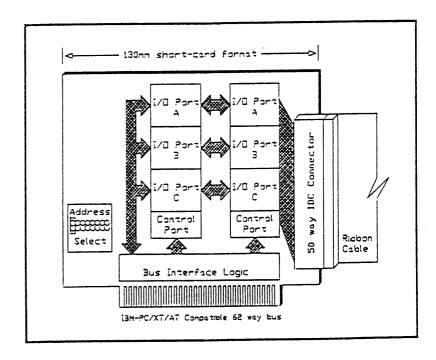
A 50 way IDC connector terminates the 48 I/O lines and 2 common lines. A screw terminal block may be attached via this connector.
