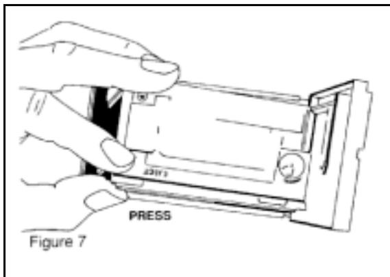
Fit a replacement cartridge, ensuring that the paper lies between the ribbon and the steel printer platen.
