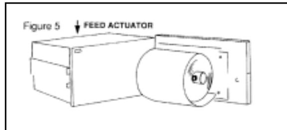
Turn the paper roll so that any loose turns are wound snugly against the roll. Close the printer door.
