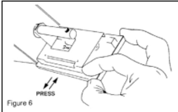
Carefully press the door and chassis in vertically opposite directions until the catch is released. Do not pull the door and chassis apart without first releasing the catch.
