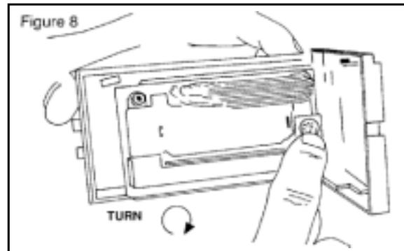
If there is some paper protruding from the front of the printer mechanism, ensure that it will pass clearly through the guide channel and past the tear bar before snapping the chassis shut against the back of the door.
