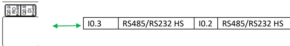
1. I0.3: If this switch is ON, the RS485/RS232 HS switch must be set to OFF. Being in ON mode it enables I0.3.
