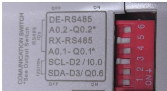
\*I2C switch serigraphy is turned around. It should be: (SDA-D2 , SCL-D3). RX-RS485 should be RE-RS485
