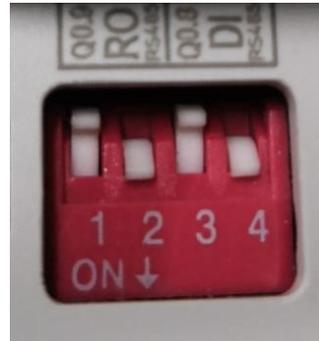
NOTE: Although in the TOP ZONE serigraphy it is shown Q0.9 & Q0.8 pins, in the reality they are I0.3 I0.2 pins respectively. Additionally although the serigraphy only is expressed for the RS485 it is also the same for the RS232. So if it is desired to enable any of the Hardware Serial connection this is the function of these switches. See chapter 8 for more information
