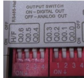
**RIGHT ZONE.** The right zone configures the outputs. If the switch is set to “ON” the Q0.X will have the behaviour of a digital output. If it is set to “OFF” it will be analog. There is also a switch for switching between Half and Full Duplex. It is “ON” for Half Duplex and “OFF” for Full Duplex.
