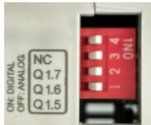
For the Relay Shield if a switch is set to ON, it can only act as Digital Output. If it is set to OFF it can only act as an Analog Output.
