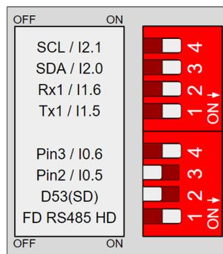
**4. SCL/I2.1:** Choosing between SCL or the input I2.1. If this switch is ON, it enables the I2.1 input and disables the SCL. If this switch is OFF, it enables SCL and disables I2.1.
