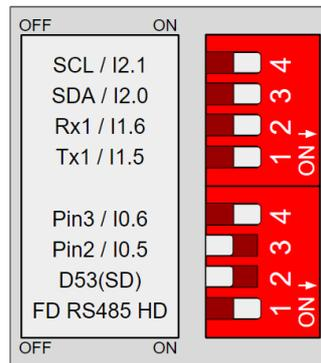
**4. SCL/I2.1:** Choosing between SCL or the input I2.1. If this switch is ON, it enables the I2.1 input and disables the SCL. If this switch is OFF, it enables SCL and disables I2.1.
