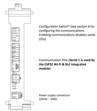
${\sf SS: Chip \, Select \, pins. \, These \, pins \, can \, act \, as \, {\sf TTL}, \, so \, they \, can \, work \, for \, the \, {\sf Chip \, Select \, pin \, of \, any \, device.} }$
