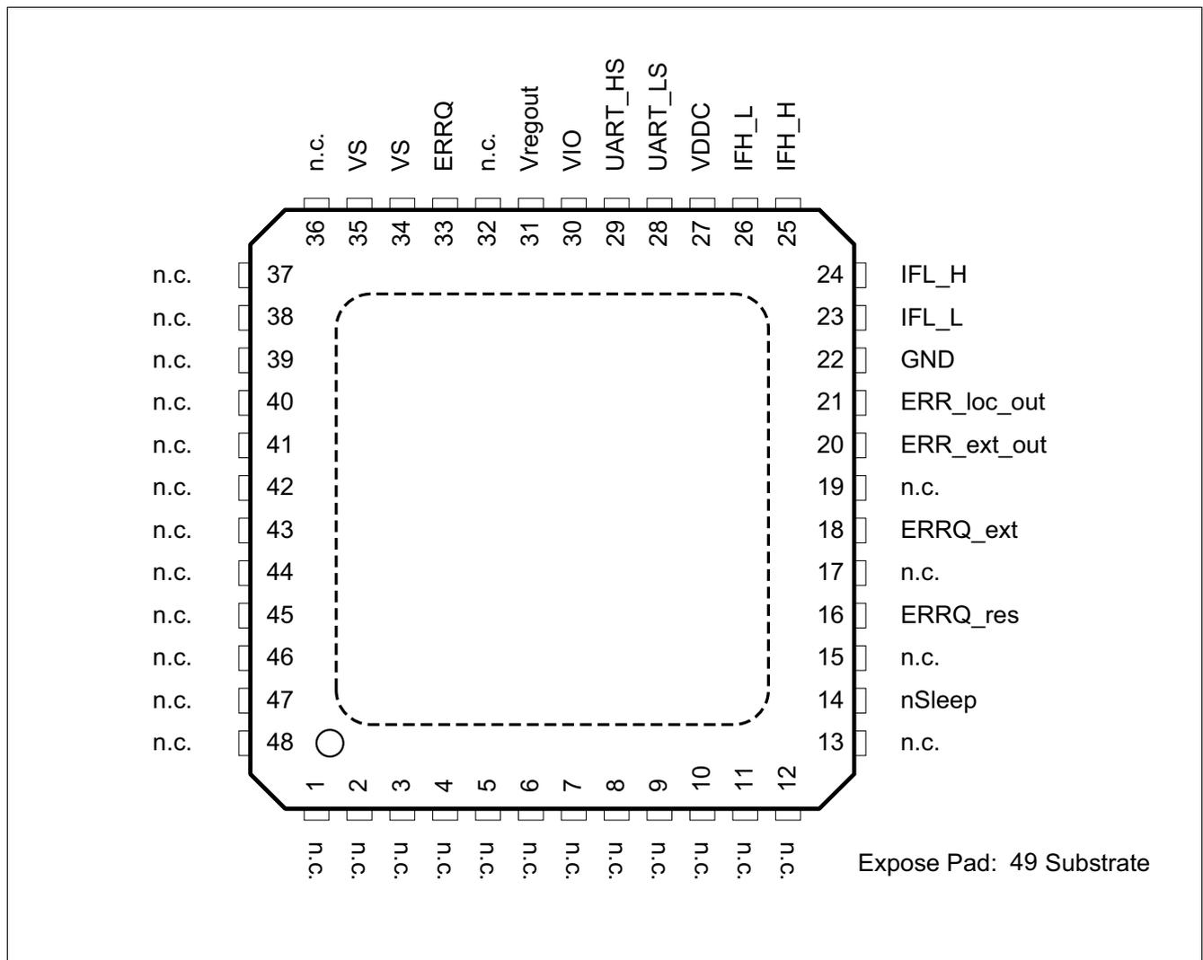
Figure 2-1 Pin configuration
