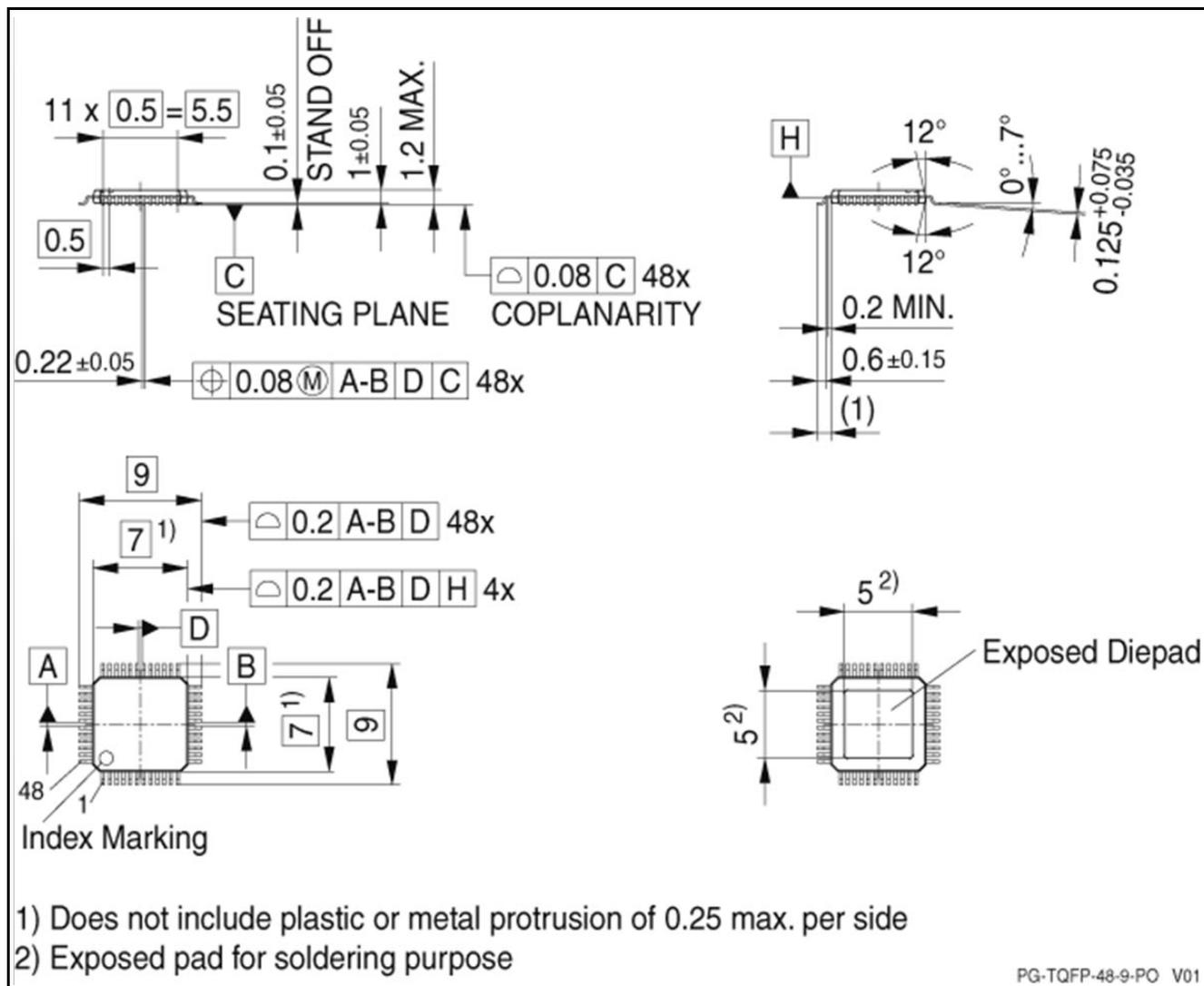
Figure 3-1 Package outlines and footprint PG-TQFP-48
