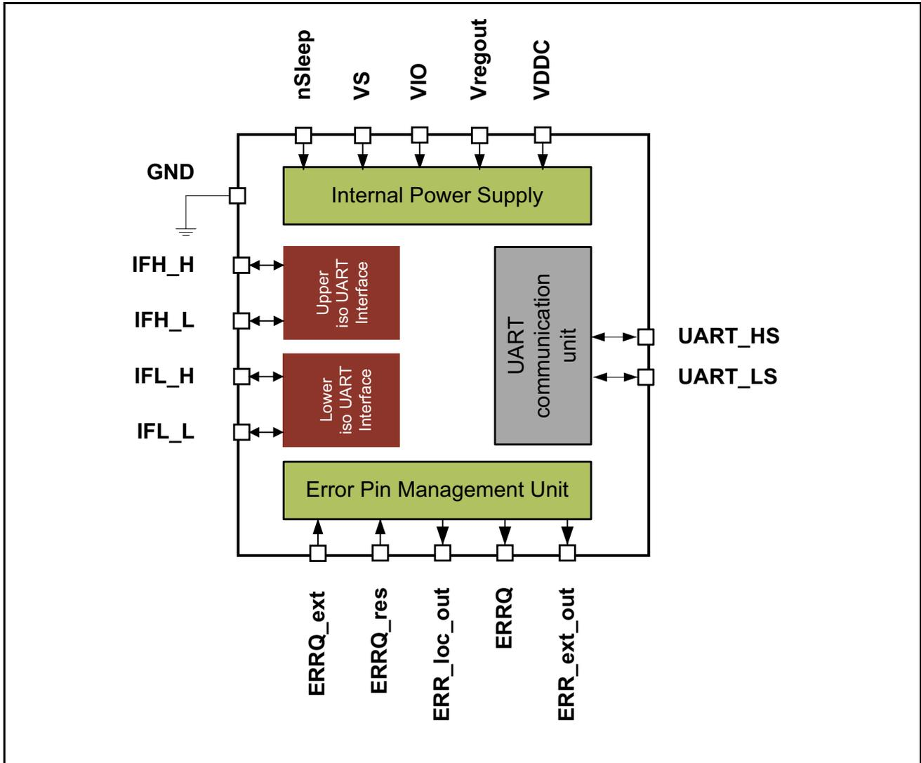
Figure 1-1 Block diagram
