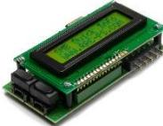
SMBus Reader                               | 100122                               | Simple read out of SMBus batteries data. No external power supply required. 5way blade connector and RS232 interface.                                                                                                           |
