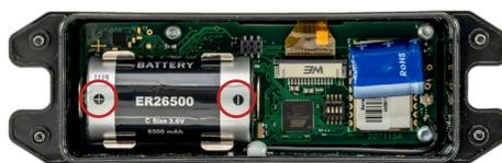
2. Insert the 3.6 V lithium battery. Verify the battery's positive and negative terminals align to the positive and negative terminals as marked.
