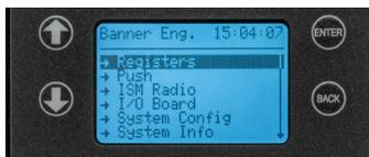
On the DXM Controller, use the arrow keys to select the **Registers** menu and press **ENTER**.
